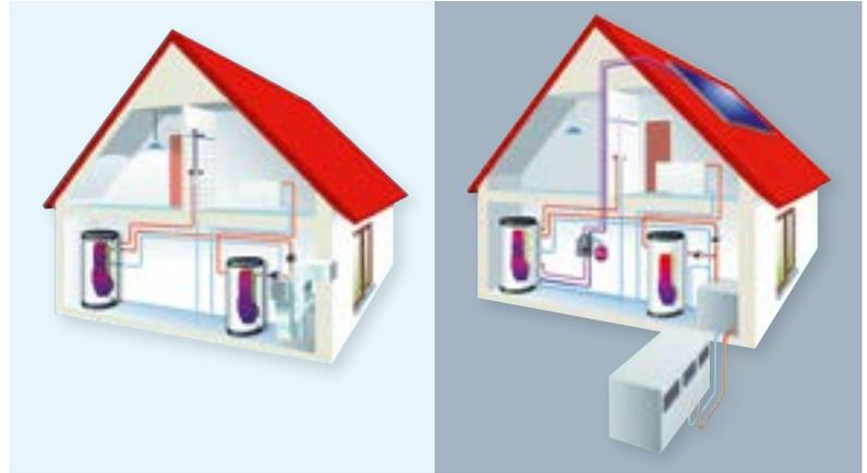
FIGURE 1: Air/water heat pumps for installation indoors (left) and outdoors (right).
